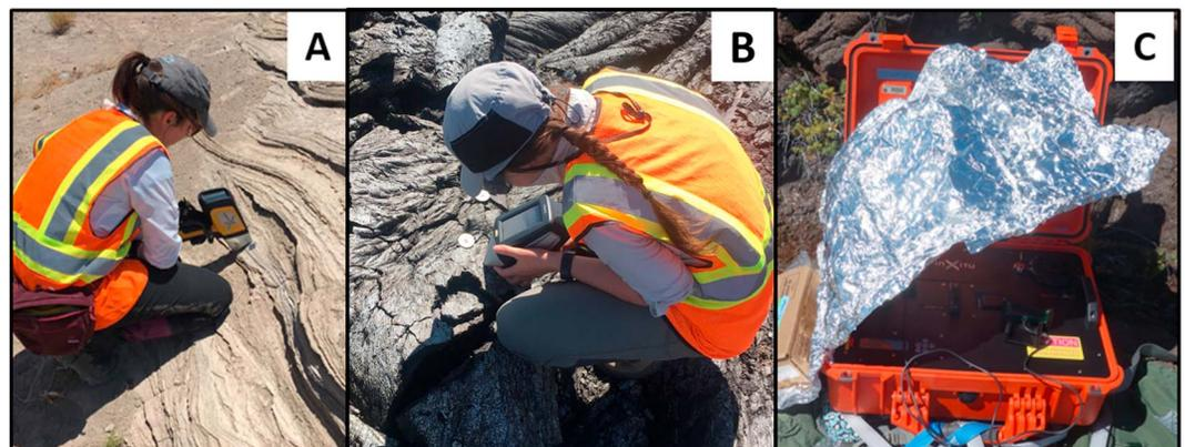
**Figure 8.** The field portable instrumentation available to the RIS<sup>4</sup>E crewmembers for in situ chemical and mineralogical analyses are shown. (a) The XRF spectrometer is handheld and acquires geochemical data with a 60-s data collection time. (b) The LIBS instrument is also handheld and provides data on the same time scales as the hXRF. (c) The XRD provides both mineralogy and chemistry information after longer integration times and some sample preparation.
