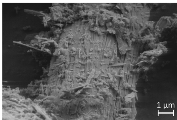
Figure 9. SEM image showing a grain of the baked and darkened antigorite dust (Fig. 7E) acquired using SE2 with 2.5 keV. While most of the particles are smaller than 10 \mu\text{m} , a small proportion of them are less than 100 \mu\text{m} along a single axis. Additional SEM images of the dust used in this study are available in the Supplemental Materials.
