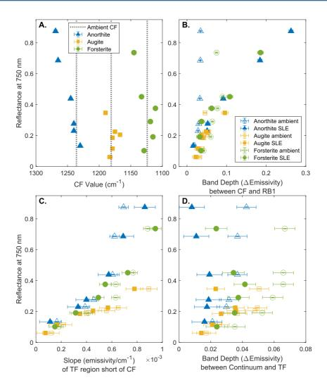
**Figure 3.** Variation of the Christiansen Feature (CF) value position (a), first Reststrahlen band depth (b), slope of the transparency feature (TF) region at shorter wavelengths/longer wavenumbers than the CF (c), and band depth from a continuum at the TF (d) compared to albedo per mineral.
