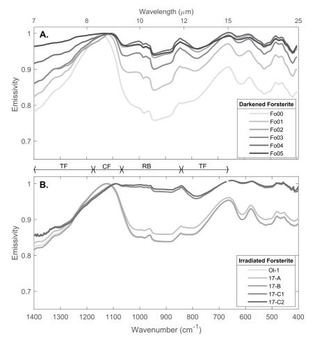
**Figure 4.**  $<32 \mu m$  carbon-darkened forsterite (a) and laser-irradiated forsterite (b) MIR emissivity spectra measured under simulated lunar environment conditions with a gray-scale to indicate pure forsterite to most "weathered." Both sets of spectra show a loss of spectral contrast, and a shift in the Christiansen Feature position to a longer wavelength with increasing npC/ irradiation. Regions of investigated features are labeled.
