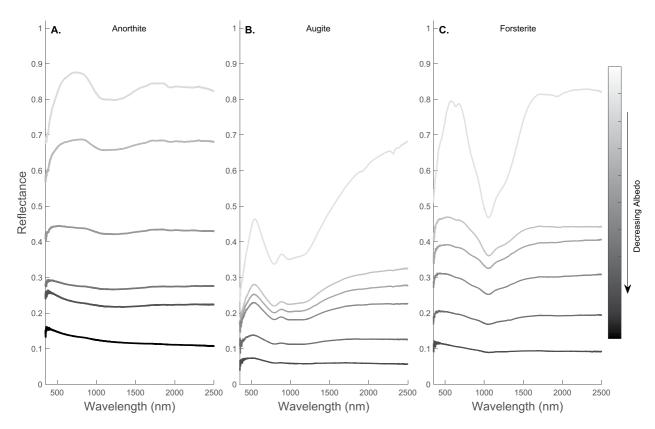
**Figure 1.** VNIR reflectance spectra of  $<32 \mu$ m anorthite (a), augite (b), and forsterite (c) darkened from pure (gray) with increasing amounts of npC to the lowest albedo (black). Overall reflectance decreases, and spectral features are lost with increasing npC addition; however, no reddening is observed likely due to the large npC particle size.
